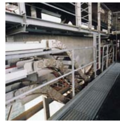
SR310 plastic chains and BS4500 stainless steel chains applied to "Oresund Bridge" between Sweden and Denmark.
